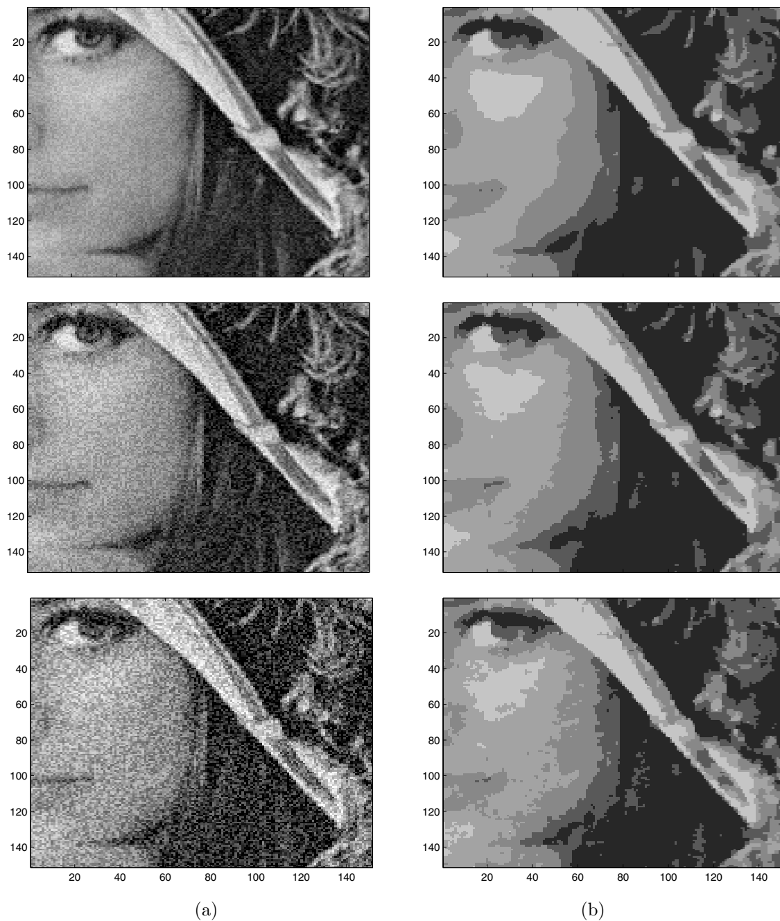
FIGURE 9. Noisy images (a) and 5-classes ( C = \{29; 71; 117; 146; 184\} ) classified images obtained using the topological method applied to the improved restoration method (b), for different levels of noise (top: SNR = 20 ; middle: SNR = 15 ; bottom: SNR = 10 ).
