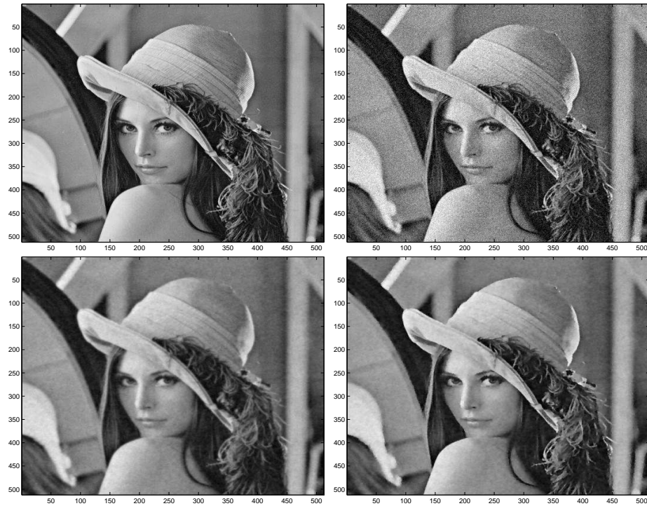
Figure 2: Top left: initial Lena image ( 512 \times 512 pixels), top right: noisy image ( \text{SNR}=17 ), down left: restored image using an homogeneous diffusion method ( \text{SNR}=27 ), down right: restored image using topological gradient method ( \text{SNR}=29 ).
