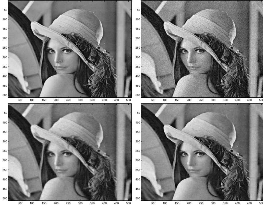
Figure 1: Top left: initial Lena image (512×512 pixels), top right: noisy image (SNR=17), down left: restored image using the linear diffusion method (SNR=23), down right: restored image using the nonlinear diffusion method (SNR=27).
