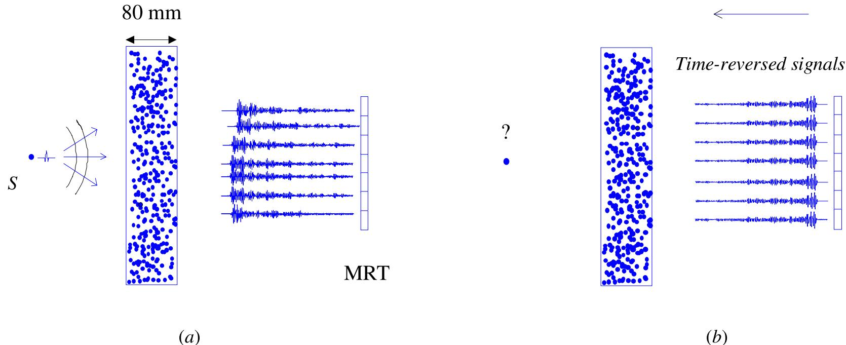
Experimental set-up for a time-reversal experiment through a multiple-scattering medium:
