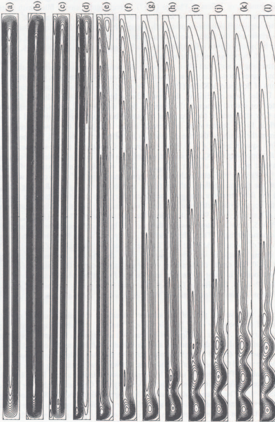
Fig. 12. Streamline patterns for Gr = 3 \times 10^3 and several negative Reynolds numbers: (a) -67 , (b) -167 , (c) -333 , (d) -500 , (e) -667 , (f) -10^3 , (g) -1.333 \times 10^3 , (h) -2 \times 10^3 , (i) -3.333 \times 10^3 , (j) -5 \times 10^3 , (k) -6.667 \times 10^3 , (l) -10^4 .
