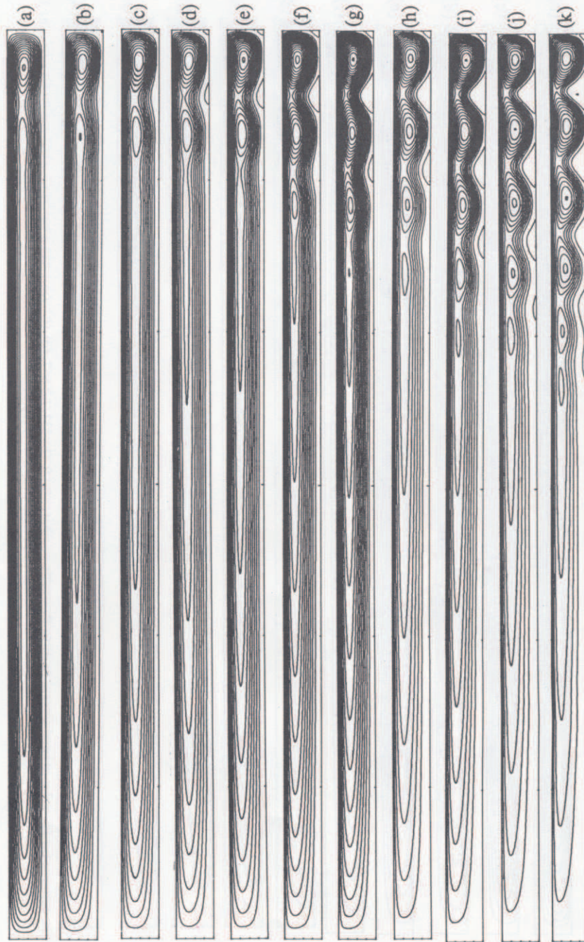
Fig. 11. Streamline patterns for Gr = 6 \times 10^3 and several positive Reynolds numbers: (a) 67, (b) 333, (c) 667, (d) 10^3 , (e) 1.333 \times 10^3 , (f) 2 \times 10^3 , (g) 2.667 \times 10^3 , (h) 3.333 \times 10^3 , (i) 5 \times 10^3 , (j) 6.667 \times 10^3 , (k) 10^4 .
