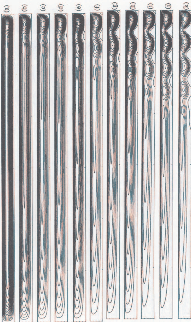
Fig. 10. Streamline patterns for Gr = 3 \times 10^3 and several positive Reynolds numbers: (a) 0, (b) 333, (c) 667, (d) 10^3 , (e) 1.333 \times 10^3 , (f) 2 \times 10^3 , (g) 2.667 \times 10^3 , (h) 3.333 \times 10^3 , (i) 5 \times 10^3 , (j) 6.667 \times 10^3 , (k) 10^4 .
