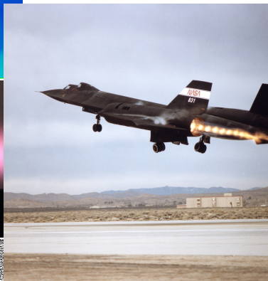
Dryden Flight Research Center EC92-1284 Photograph SR-71B take-off with "shock diamonds" in the exhaust.
