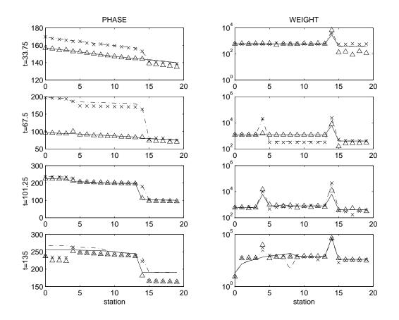
Phases (left) and densities (right) as a function of 'space' at various times (top to down) Kinetic ( $\times$ ,  $\Delta$ ) and two-phase (--, - · -) models
