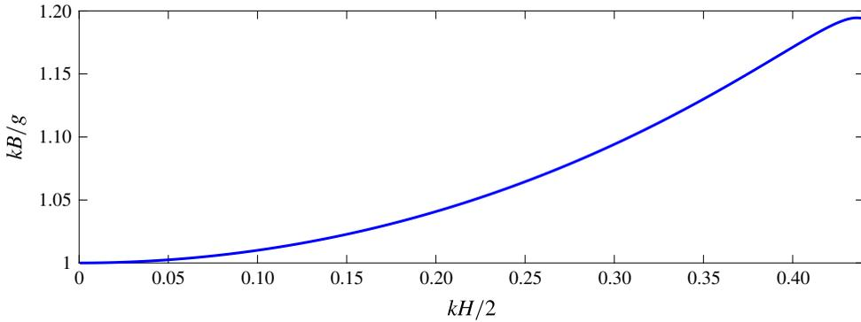
FIGURE 7. (Colour online) The Bernoulli constant in deep water as a function of the steepness.
