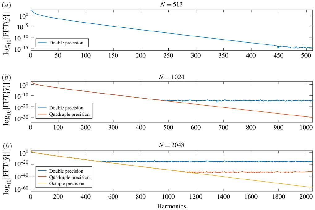
FIGURE 3. (Colour online) Decay of the Fourier coefficients for  $\varepsilon = 0.4$  and  $kd = \infty$ : blue, 16 digits; red, 34 digits; orange, 71 digits.
