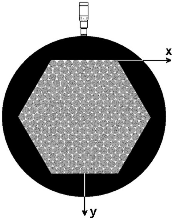
FIG. 1. Sketch of the load cell. The collection of cylinders is packed into a triangular (centered hexagonal) compact lattice, and confined into a rigid hexagonal frame. Cylinders are 8 mm in diameter. Grains are seeded with tracer particles. The displacements of the tracers are tracked as the punch is progressively moved inward.
