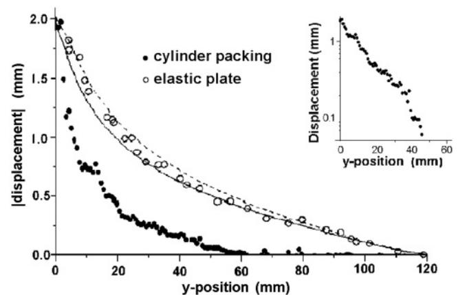
FIG. 3. Displacement amplitude, measured along the load axis  $Oy$  ( $\bullet$ , discrete piling;  $\circ$ , continuous plate) and elastic predictions for various Poisson moduli in a plane strain modeling (continuous line,  $\nu = -0.9$ ; dashed line,  $\nu = 0.5$ ). In inset, semilogarithmic plot of the displacement amplitude as a function of  $y$ .
