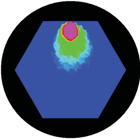
FIG. 4. (Color online) Same data as Fig. 2. Displacement amplitude as a function of the position  $(x,y)$ , coded in color levels. The contours corresponding to displacements of equal amplitude are approximately elliptic.
