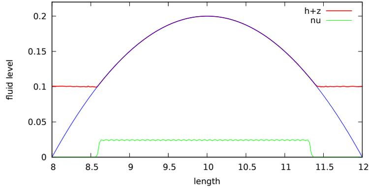
**Fig. 1.1** Bump problem:  $D = (8, 12)$ ,  $t_F = 400$ , 60 elements,  $N = 4$ ,  $\alpha = 1$ ,  $\beta = 10$ ,  $h_{\text{thres}} = 10^{-4}$ . EVM solution and entropy viscosity at time  $t_F = 400$ .
