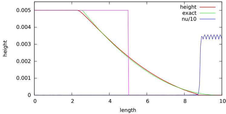
**Fig. 1.4** Dam break problem:  $D = (0, 10)$ ,  $t_F = 120$ , 60 elements,  $N = 4$ ,  $\alpha = 2$ ,  $\beta = 20$ ,  $h_{\text{thres}} = 10^{-6}$ . EVM and exact solutions, entropy viscosity at  $t_F = 11$ . The initial condition is also shown.
