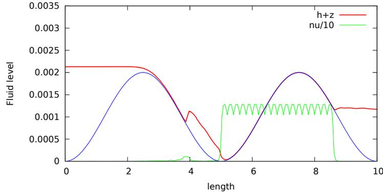
**Fig. 1.5** Dam/bump problem:  $D = (0, 10)$ ,  $t_F = 600$ , 60 elements,  $N = 4$ ,  $\alpha = 1.5$ ,  $\beta = 30$ ,  $h_{\text{thres}} = 10^{-5}$ . EVM solution and entropy viscosity at  $t = 129$ . Initial condition:  $h + z = 0.003$  if  $x < 2$ ,  $h = 0$  if  $x > 2$ .
