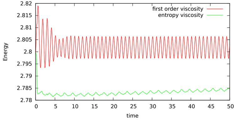
**Fig. 1.3** Cup problem: Time-variations of the total energy for the solutions obtained with the entropy viscosity and with the first order viscosity
