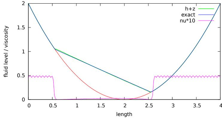
**Fig. 1.2** Cup problem:  $D = (0, 4)$ ,  $t_F = 50$ , 60 elements,  $N = 4$ ,  $\alpha = 1$ ,  $\beta = 10$ ,  $h_{\text{thres}} = 10^{-3}$ . EVM and exact solutions, entropy viscosity at time  $t_F = 50$ .
